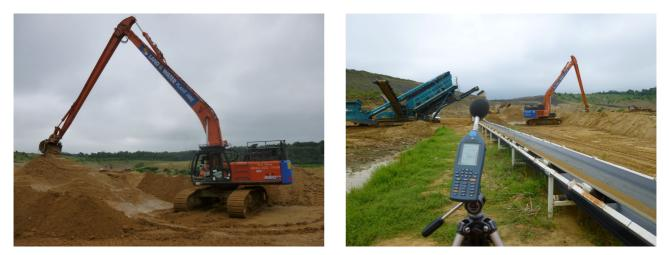
Some examples of tracked excavators where the manufacturer's quoted sound power levels are at or below 104 dB  $L_{WA}$  include the Komatsu HB365LC/NLC-3, Hitachi ZAXIS 210 and SANY SY500H.
